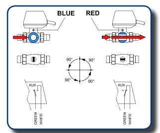
Utilisable fluids: water or liquids compatible with PTFE and EPDM. Before installing the valve be sure that no solid residues, like welding or threading residues, remain in the hydraulic circuit.
