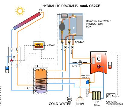
Circulator P1 in the solar circuit is ON only when T1 — T2 ≥ 5 °C
