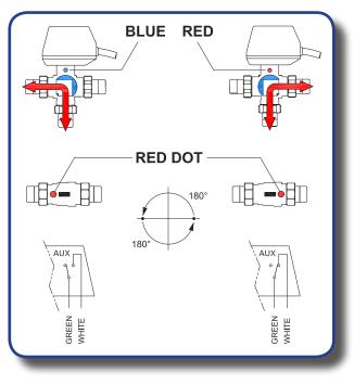
SUITABLE FOR WATER OR LIQUIDS COMPA-TIBLE WITH PTFE AND EPDM. PRIOR TO IN-STALLATION, ENSURE THAT THE HYDRAULIC CIRCUIT IS CLEANED OF SOLIDS SUCH AS WELDING OR THREAD RESIDUES.
